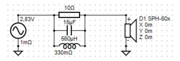
Coilferrit core coil for best value/money , resistance should be no higher then 0,5 ohmsCapacitorbipolar, 50VAC typeResistorany 10 Watt type
